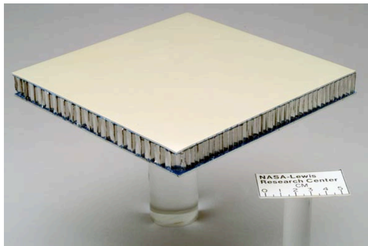
Glass aluminum reinforced (GLARE) honeycomb composite sandwich structure.
