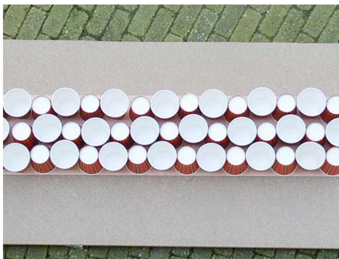
Coffee cup - honeycomb sandwich structure.
