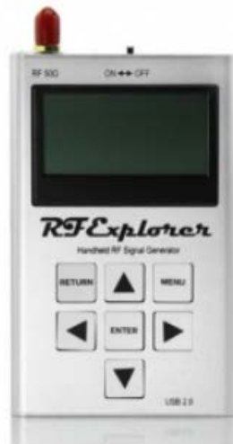
Figure 1: The RF Explorer Signal Generator. Capable of producing replica RF signals that can simulate embedded ‘bug’ devices
