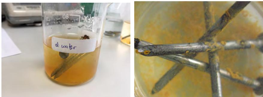
Tests using **Pinnacle “yellow zinc” washers** with deionised or demineralised water produced small bubbles of gas on the surface of the washers. There were visible changes to these washers.
