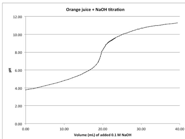
Titration of commercial orange juice with 0.1000 M NaOH
