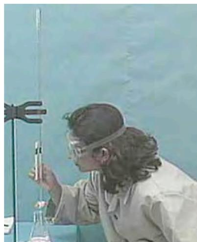
Correct (✓): eyes are level with the liquid surface
