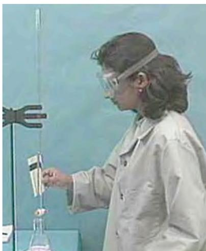
Incorrect (✗): eyes are not level with the liquid surface
