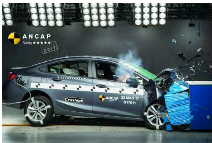
Holden Astra (May 2017 – onwards) frontal offset test at 64km/h. Photograph © Australasian New Car Assessment Program (ANCAP). http://www.ancap.com.au/safety-ratings/holden/astra-25ad9072-b3da-4fb0-863e-37045a3cac7c/4fc8d4/images-and-video
