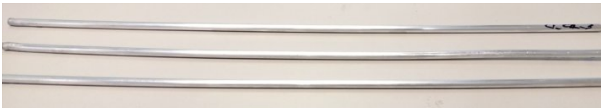
Figure 3: Typical defect free extruded samples of different compositions. The total length of the extruded product is about 450 mm.
