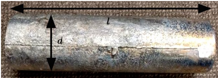
Figure 1: Photograph of a direct chill cast Al alloy. Length (l) = ~200mm, diameter (d) = 80mm.
