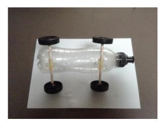
9. Place car on its wheels, and push roll to make sure that the car rolls in a straight line – if it veers to one side, take the affecting axle off and reattach inline
