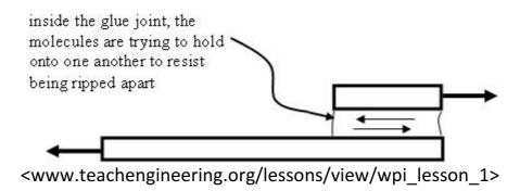
**Shear strength** – the shear load required to break an object or joint.
